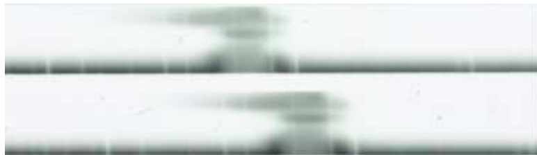
Fig. 1. General appearance of the H-alpha line in the studied spectrogram in two polarizations corresponding to combinations of Stokes parameters I+V and I-V.
